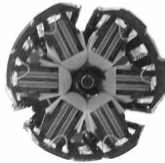
Fig.9 Resistor units of insulating frame
